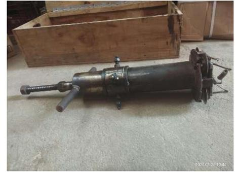
CPMCGSI special fabricated tool for inner pipe cold cutting method. Special tool has been used one time to cut a jet nozzle mixer inside the tank where access is impossible and where cold cutting is required for safe cutting/demolition. Jet mixer nozzle was allowed to be left inside the tank though.
